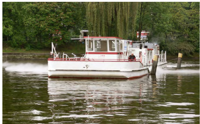
Fig. 15: Combined sewers. Fig. 16: In order to combat the fish die-offs the aeration vessel is supplying surface water with oxygen.
